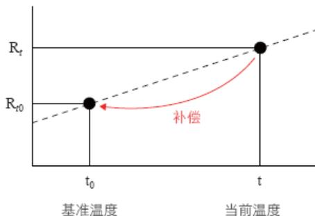
$$R_{t_0} = \frac{R_t}{1 + \alpha_{t_0}(t - t_0)}$$
